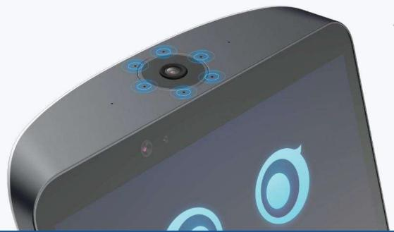
The 6-MIC microphone array has **over 97% speech recognition accuracy** in noisy environments of 75dB.
