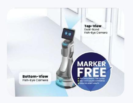
By harnessing Qualcomm's GPU/DSP chips and cutting-edge deep learning, 365NovaBot ensures real-time positioning even amid changing angles and lighting conditions. Say goodbye to localization errors and hello to stable and efficient robot operations. Greater adaptability to diverse scenarios
